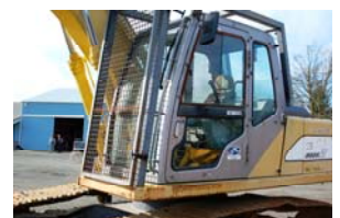
Inadequate Safety Shield
