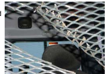
Damage to the Safety Shield in Front of Cabin
